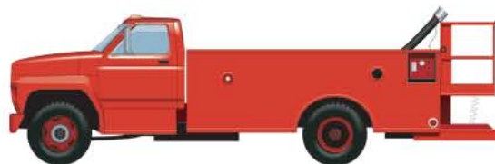
camion M vide-toilette M lavatory truck camión M sanitario Toilettenwagen M botte F igienica semovente
